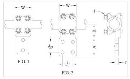
Print This Page Download As PDF Pad Width **Catalog Number** Fig. No. Pipe Size (NPS) A (in) B (in) W (in) T (in) J (in) Weight (lb) ATF-60-4A 2 2 1/2 3 3 3 1/8 3 1/2 5/8 1/2 3.1
