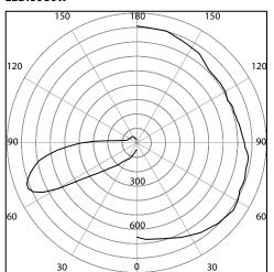
\* Photometric distribution is based on Lexalite Lindy 424 per DLC specifications in a Type V distribution.
