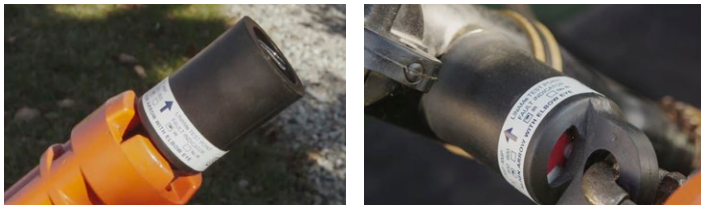
Easily attach the SEL-TPR to capacitive test points with a single hot stick.
